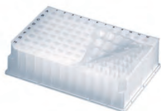
Collection plate, showing 96-position closing mat, 5042-1389
